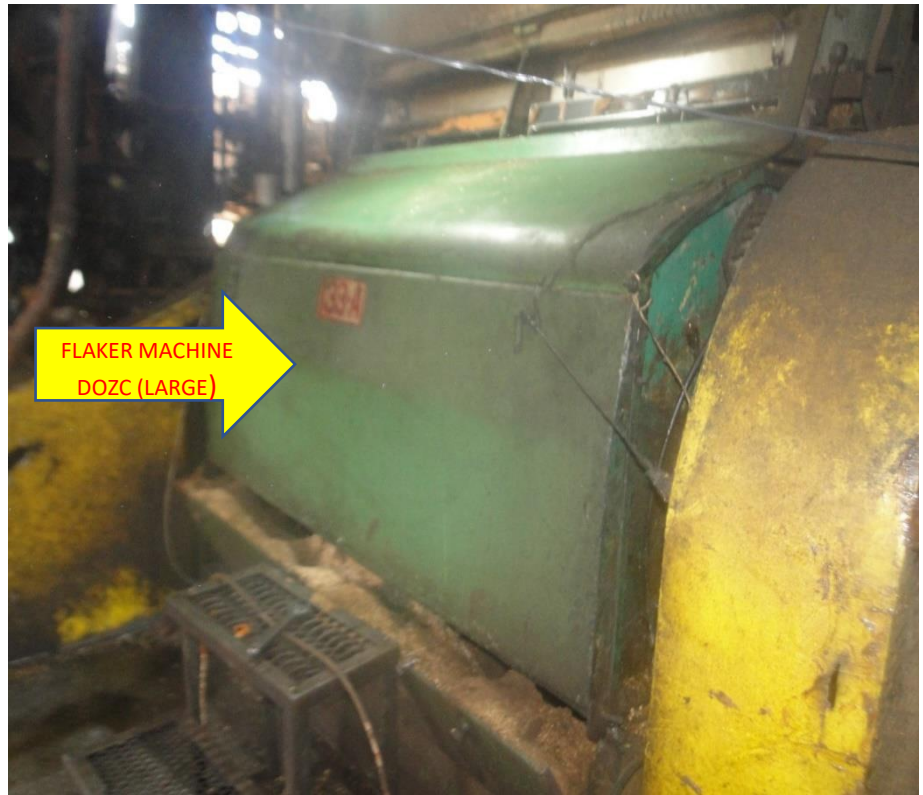
Flaker Roller DOZC size 800 mm diameter x 2000 mm length
